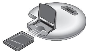
*Open the small compartment on a back of BeoSound 2 to insert a memory card.*
